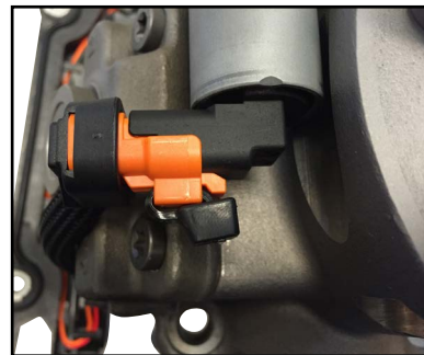
Connector Locked with Tie Strap Secured
