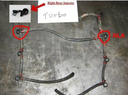
The original right rear injector return line tee is no longer available. In this kit we have substituted a double return tee, with a plug and clamp.
